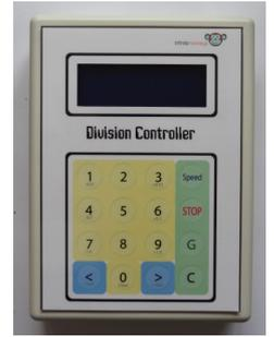
First the case should be drilled to take the keypad and the keypad mounted on spacers to set the buttons edges flush with the case (the buttons are slightly rounded and it's this slight protrusion that will determine how the keypad 'feels').
