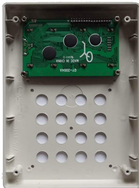
Fig 3 – Case internals with LCD fitted.
